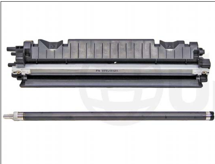
15. Remove the magnetic roller assembly.
